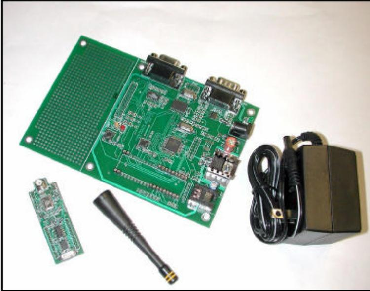
Transmitting and receiving data at 20kbps in the unlicensed 900MHz band, the **CANRF** will connect CAN nodes up to 250' apart. Power output is set at 0.25mW into 50 ohms (-1.25dBm) but can be adjusted up to 0.75mW if an inefficient antenna keeps the signal down below the FCC Part 15 regulations.
